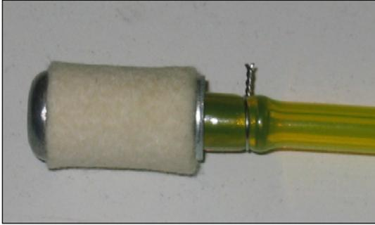
Now place a 6mm flat washer on the felt pendulum and connect it with the Tygon tube. This will prevent slippage of the felt body. Then secure the Tygon tube connections with wire. Again, check for leak tightness.
