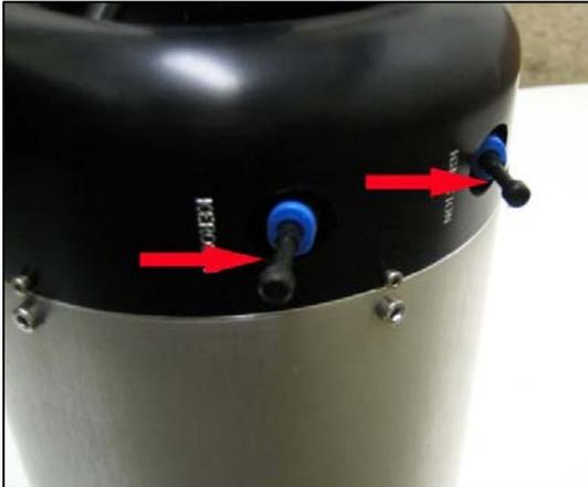
When the turbine is not used or returned to the factory, the kerosene and propane joints must always be sealed. Please use included plugs. Miniscule particles can clog kerosene tubes and fault free operation of the turbine cannot be guaranteed.
