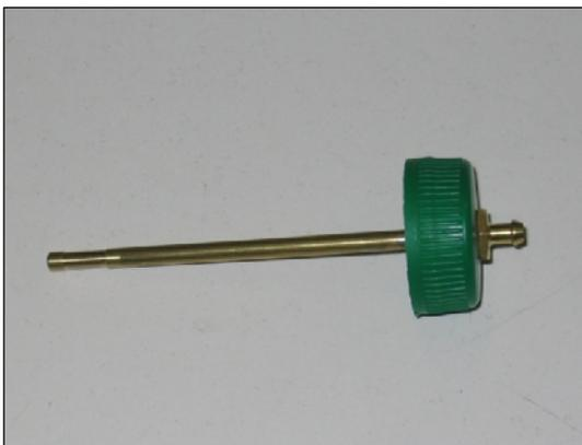
Use the included tank pendulum device and screw it together with the tank cap. Check for tightness. Cut a piece of Tygon tube with a length of ca. 120 – 150 mm. This is the ideal length for the typically used 1.5 liter and 2.0 liter Coca Cola bottles. The length of the tank pendulum, however, depends on the type of tank used. We recommend to choose the length the way that the felt pendulum lies at around 75% of the tank length.
