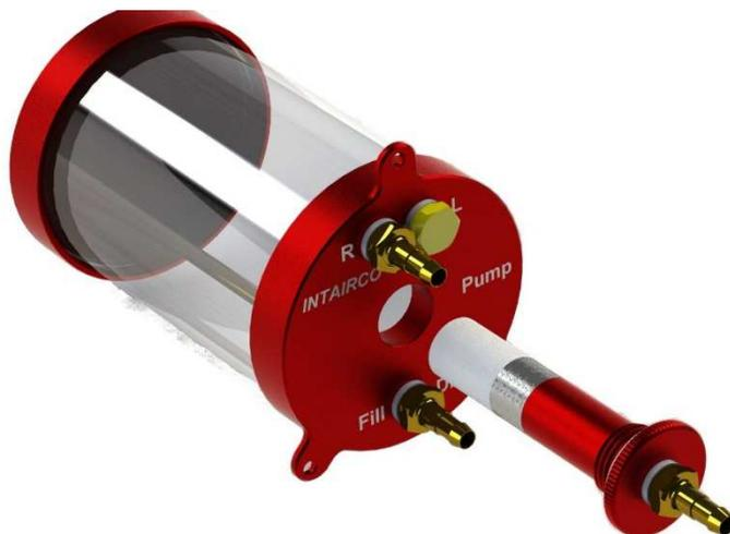
The Centre Pick-Up Tube simply unscrews from the front face of the **Super-Trap** giving access to the Super-Flow Sintered Filter. This in turn unscrews from the Pick-Up Tube Body and can be washed and blow out using an air gun from the inside.
